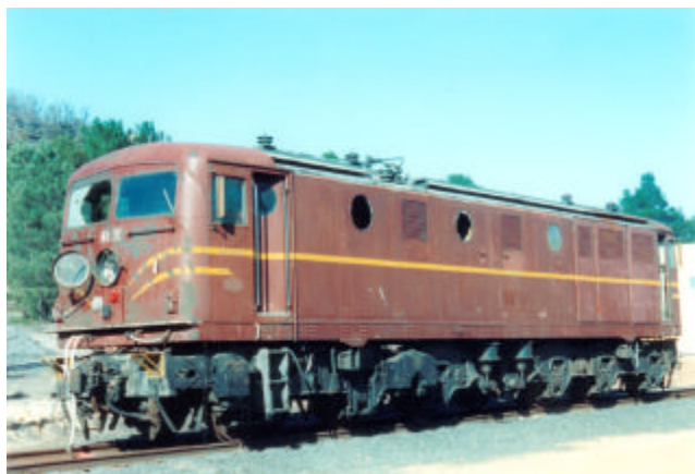
ABOVE: One of the eight 46-class units not to receive a heavy overhaul in the 1980's was 4631. This unit retained the original three-porthole configuration, along with the Stone headlights, up to its demise. Stripped of pantographs and with several windows smashed, 4631 will shortly end its days grounded on the "Lawn Cemetery" at Lithgow Maintenance Centre (John Hourigan)
