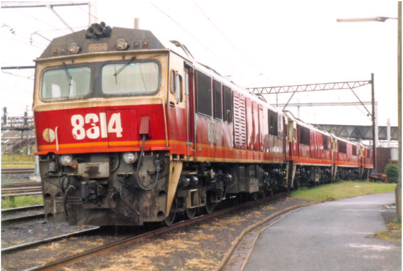
ABOVE: The electric locos were often the dirtiest on the system during the State Rail years. This was due to copper fallout from the overhead making their paint finish almost invisible! Measures to rectify this see 8614/21/46 & 39 outside ACDEP after their wash on 28 September 1993 (Greg Oates) BELOW: In 1989, 8602 received an experimental version of the FreightRail blue scheme that became known as the "stealth" livery. This unit leads candy-stripe 8649 and 4495 dead-attached on 5282 up freight through Gosford Yard on Thursday 8 November 1990 (John Hourigan)
