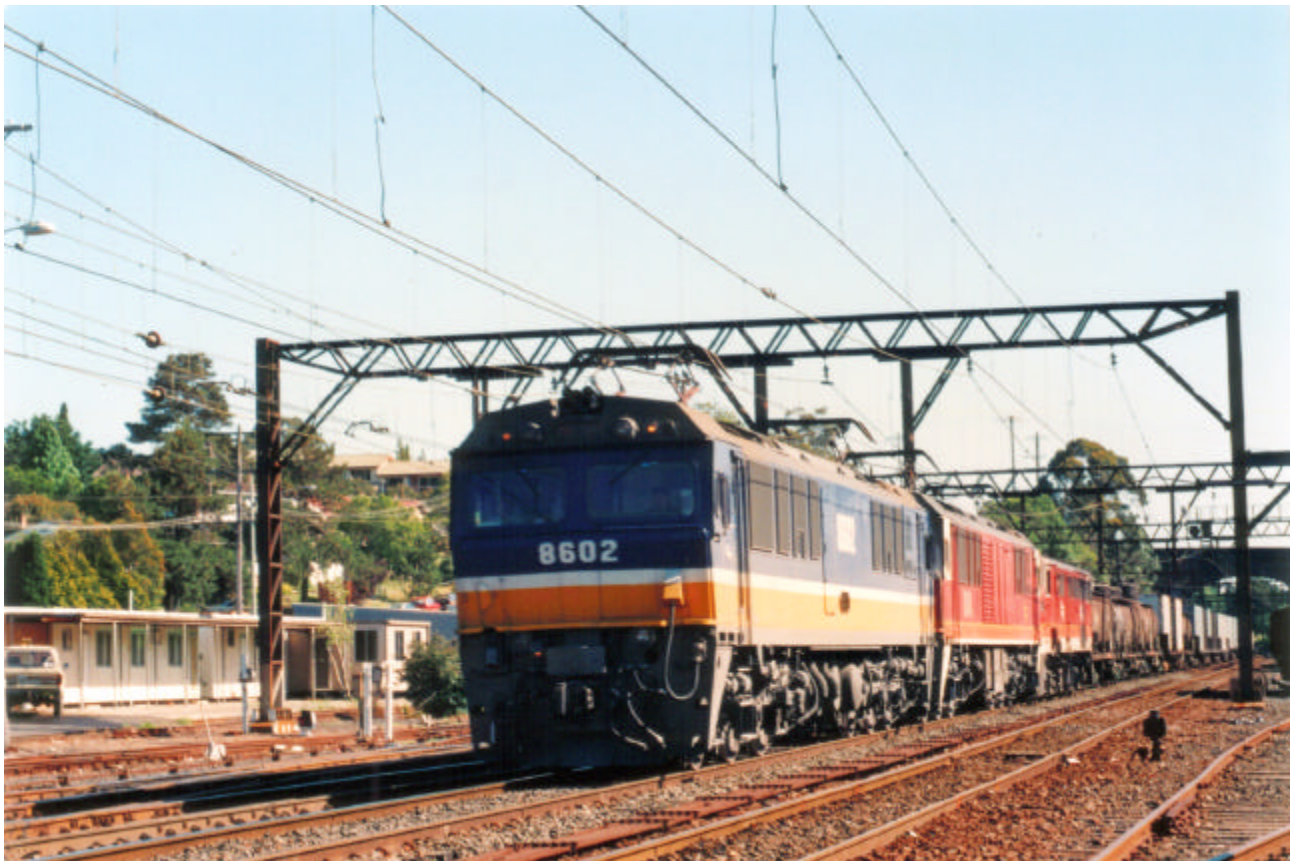
ABOVE: The electric locos were often the dirtiest on the system during the State Rail years. This was due to copper fallout from the overhead making their paint finish almost invisible! Measures to rectify this see 8614/21/46 & 39 outside ACDEP after their wash on 28 September 1993 (Greg Oates) BELOW: In 1989, 8602 received an experimental version of the FreightRail blue scheme that became known as the "stealth" livery. This unit leads candy-stripe 8649 and 4495 dead-attached on 5282 up freight through Gosford Yard on Thursday 8 November 1990 (John Hourigan)
